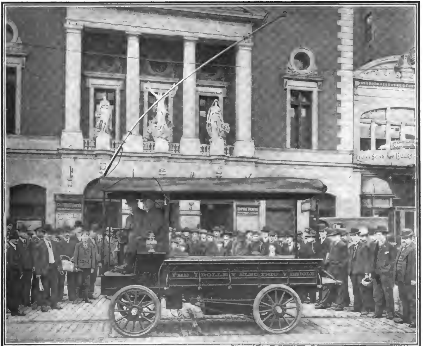
ELECTRIC WAGON, BUILT TO RUN ON CURRENT FROM TROLLEY WIRE AND INDEPENDENTLY ON STORAGE BATTERY CURRENT.
